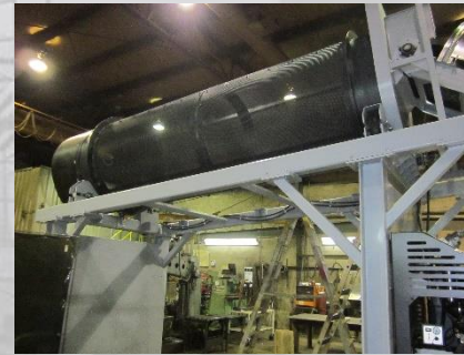
5' dia. x 16' trommel for shingle grits
