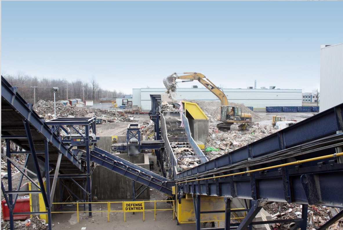
C&D recycling plant, Chateauguy QC (50 @ 60 TMPH of C&D waste)
