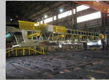
Belt conveyor 48" x 44' for anode furnace
