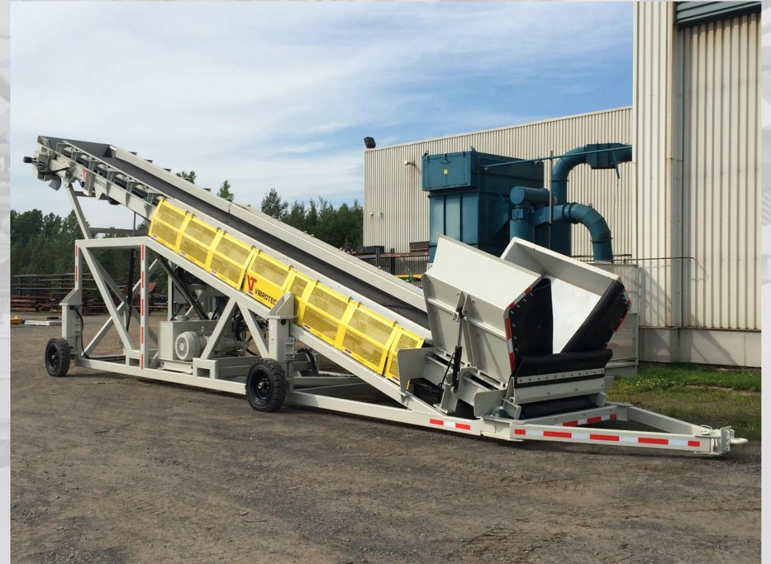
Reload conveyor, Quebec QC (48" wide, 800 TPH)
