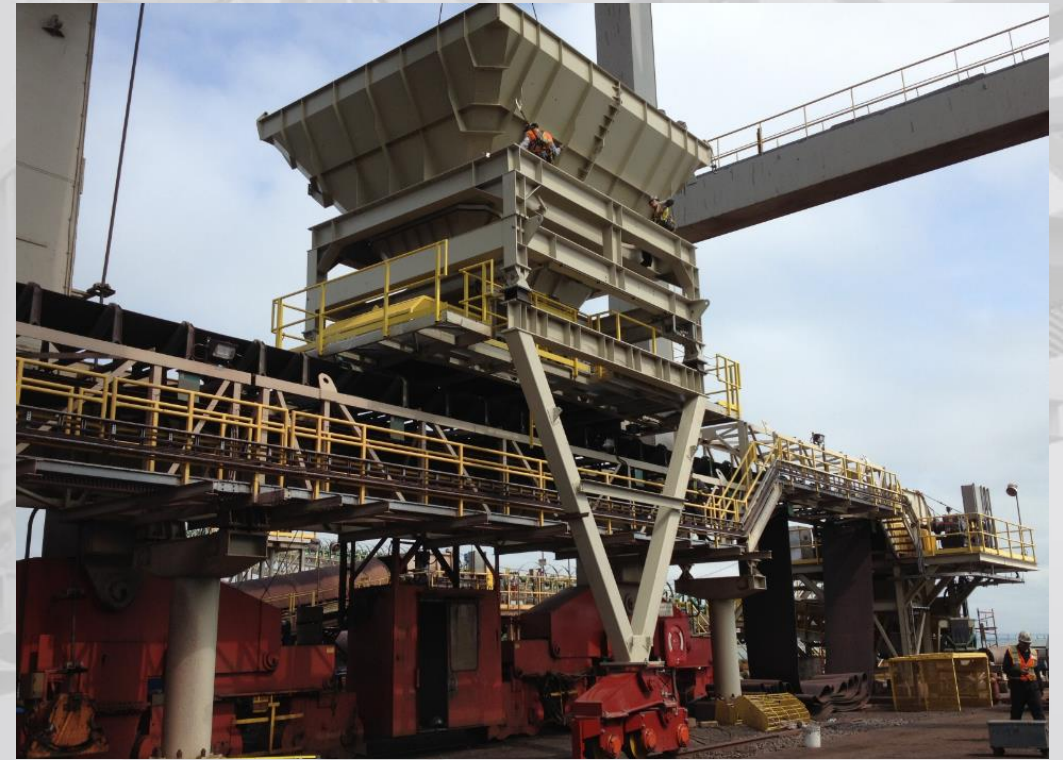
Hopper belt feeder, Beauport QC (48" wide, 3500 MTPH)
