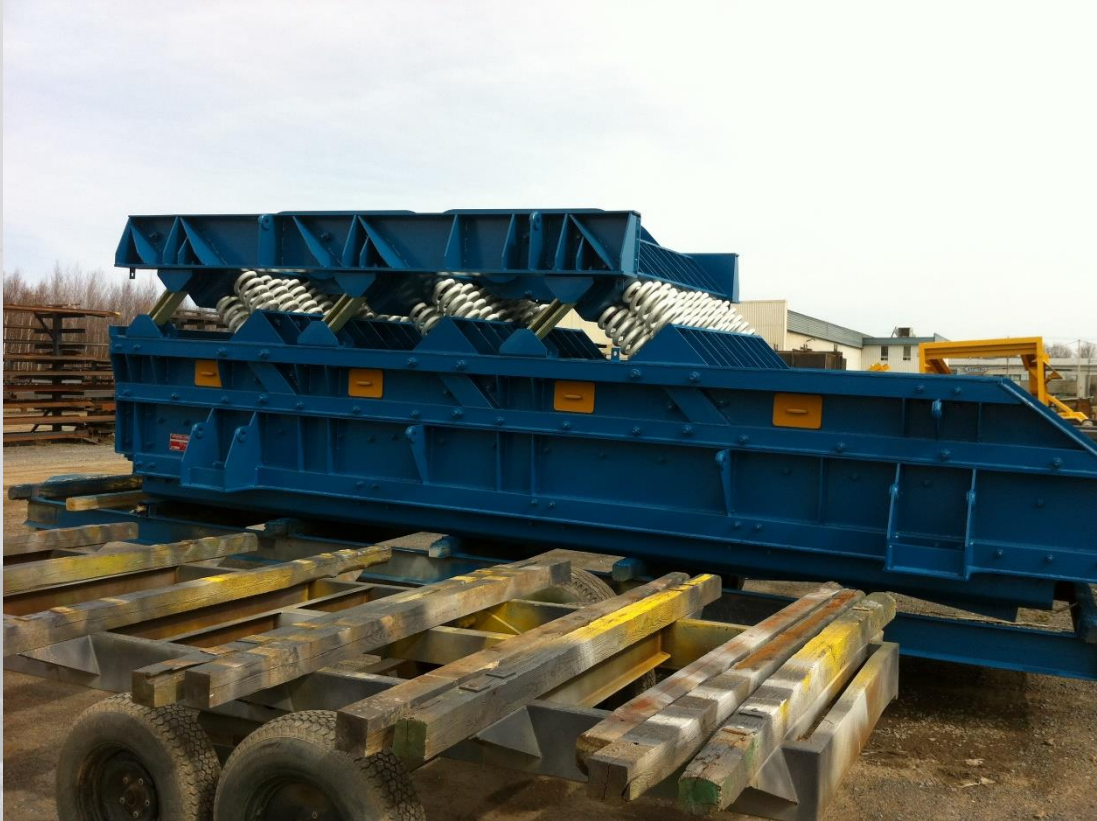
Iron ore pellets screen, Wabush QC (7' x 24', 320 MTPH)
