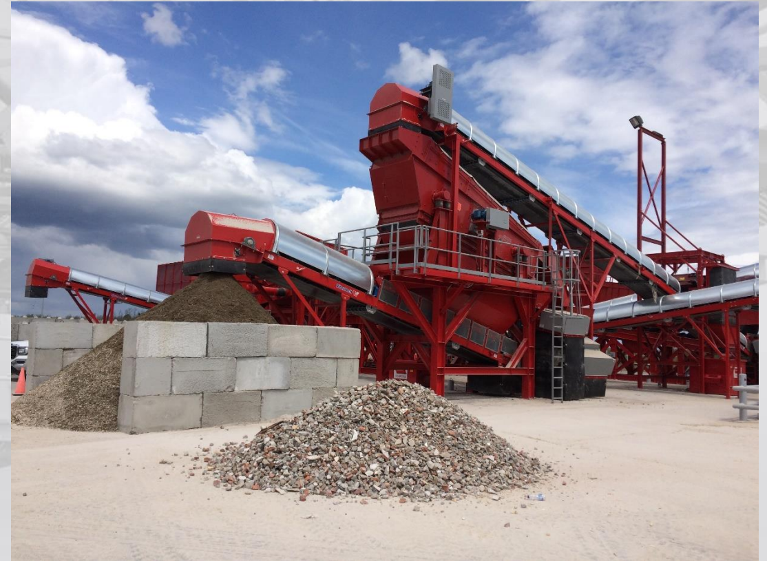
C&D recycling plant, Ottawa (50 @ 100 TMPH of C&D waste)
