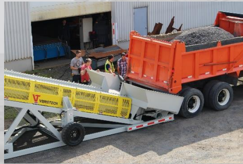
Reload conveyor test (800 TPH)
