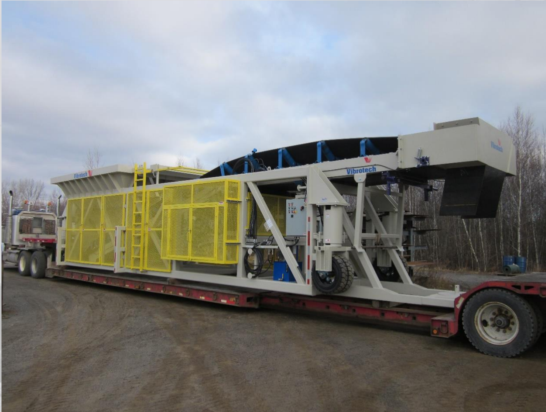
Mobile hopper feeder, Quebec QC (54" wide, 1500 TPH)
