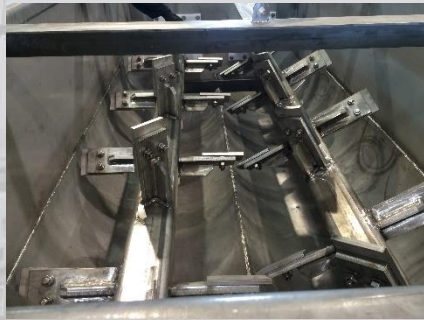
Pugmill for salt coating (750 TMPH)
