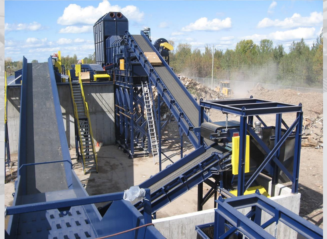
C&D recycling plant, Chateauguy QC (50 @ 60 TMPH of C&D waste)
